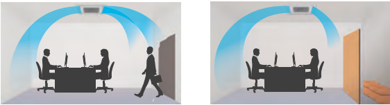
Comfortable air conditioning by preventing direct blowing of cold air and by providing swinging air flow simultaneously. Provides efficient air conditioning based on the room layout
