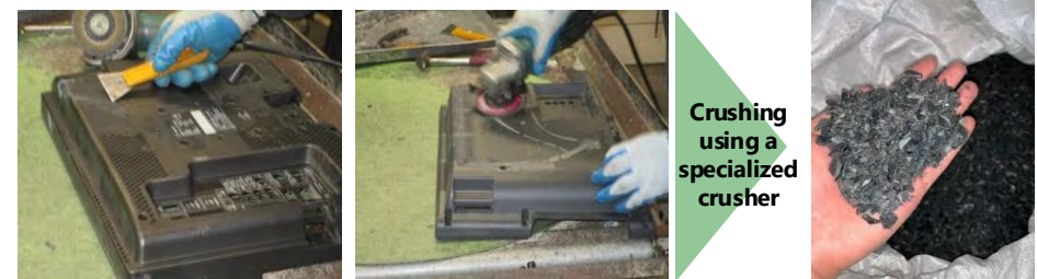
Removal of foreign substances (labels, metals, etc.) from cabinets
